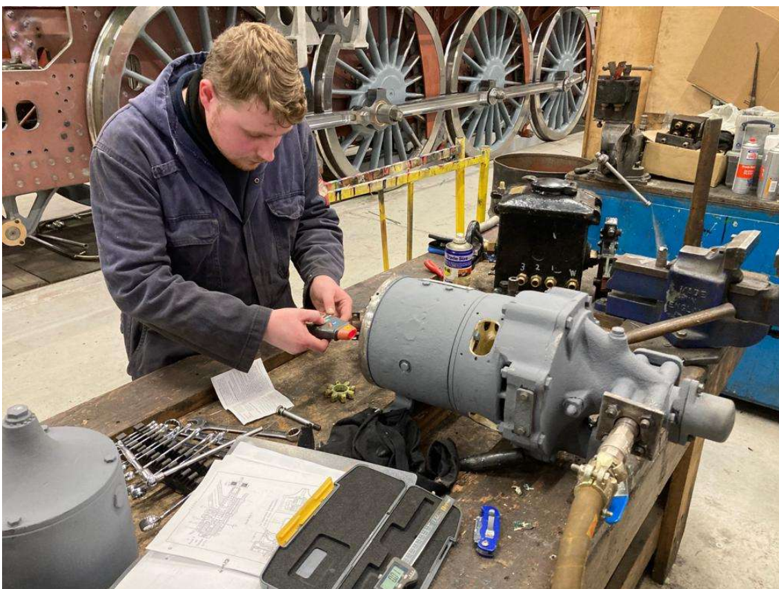
Locomotive Fitter, Ian Greenan, uses the handheld techno to check and set up the governor following overhaul of the turbogenerator.
